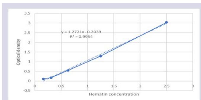
**Figure 2:** Calibration curve of haematin concentration vs optical density.
